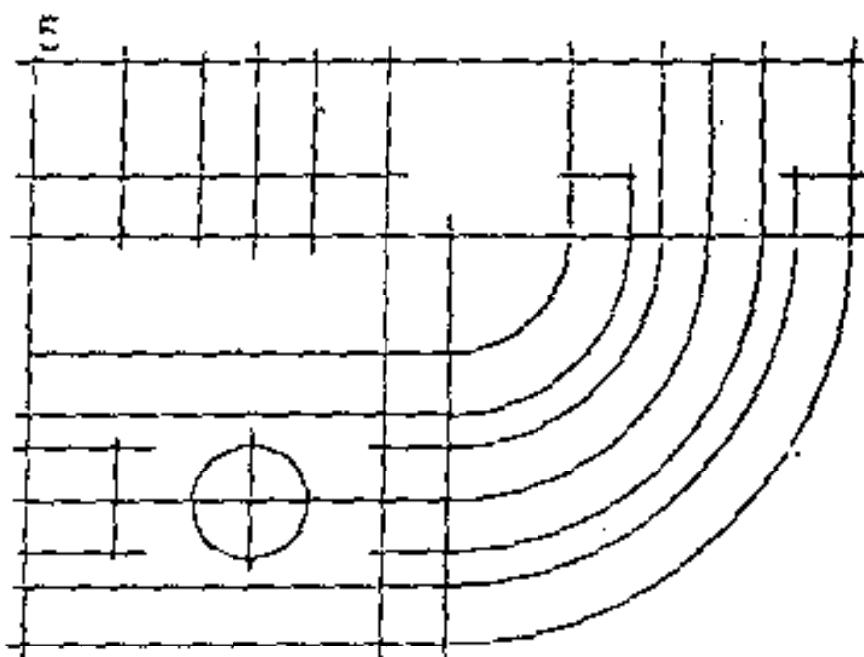
*Project detail from end view and plan into the front view*
