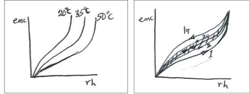
From the diagram, during sorption, the path of the curve is as shown as curve 1. It is expected that the curve will come back through the same path. However this doesn't happen in practice. Therefore curve 1a represent the desorption curve which shows that there a lagging effect called hysteresis (shaded portion) representing a lost in energy!. This effect is repeated with
