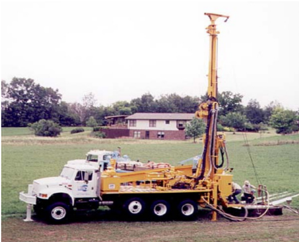
Figure 7: A typical borehole drilling rig
