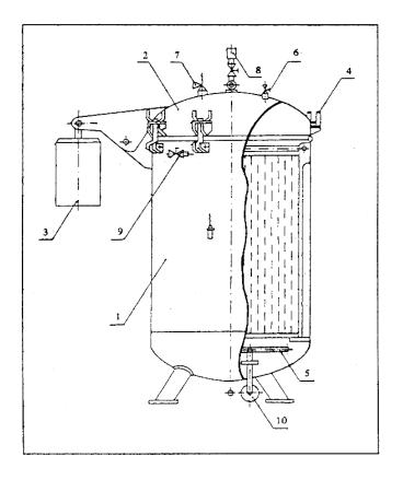
FIG.1. Retort cooker. 1. body, 2. lid, 3. counterbalance, 4. nuts, 5. heater, 6. vent, 7. relief valve, 8. pressure gauge, 9. water supplyvalve 10. steam supply valve.
