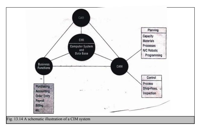
Fig. 13.14 above shows a schematic illustration of Computer-Integrated Manufacturing systems. It consists of a lot of sub-systems that are integrated into a whole. The subsystems are
