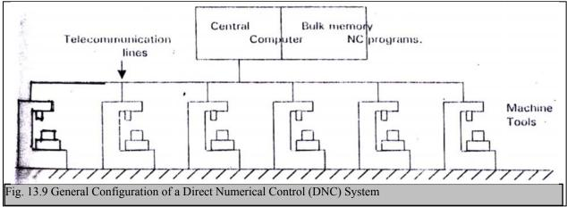
Fig. 13.9 General Configuration of a Direct Numerical Control (DNC) System
