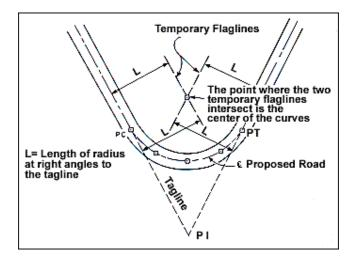
**Figure 1.**The center stake method of creating a horizontal curve is limited to use on gentle terrain with good visibility. (Redrawn from Figure 2.4-1, Darrach et al. 1981)
