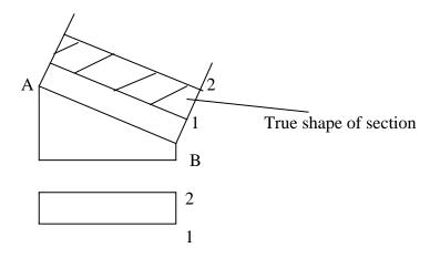
To draw the true shape of the section of the truncated hexagonal prism
