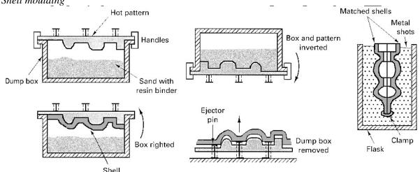
Figure 2.4: Steps in shell moulding
