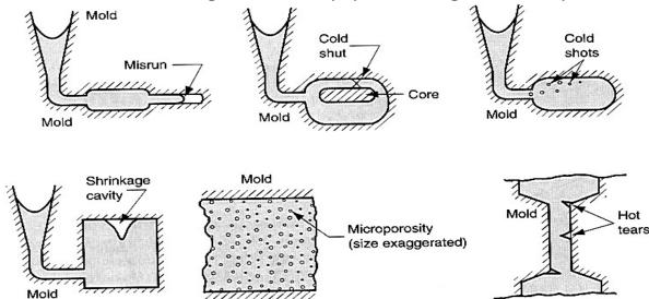
Figure 2.9: Some defects of casting
