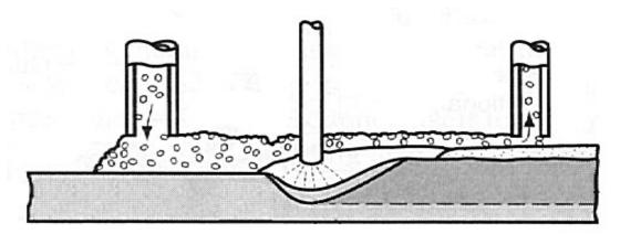
Figure 5.6: Submerged arc-welding operation.
