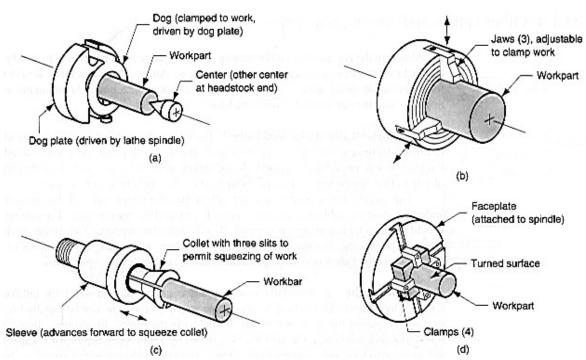
*Figure 2.17: Four Work-holding methods used in lathes:* (a) mounting the work between centres using a dog, (b) three-jaw chuck, (c) collet, and (d) face plate for noncylindrical work parts.
