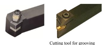
Cutting tool for straight turning
