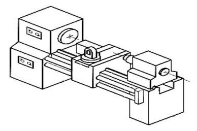
Figure 2.16: The principal components of an engine lathe
