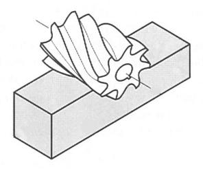
Figure 2.21: Peripheral slab milling operation
