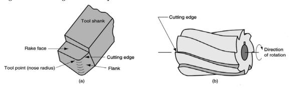
Figure 2.20: (a) A single-point tool showing rake face, flank, and tool point; and (b) a helical milling cutter, representative of tools with multiple cutting edges.
