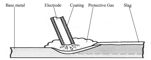
Figure 5.5: Shielded metal arc welding operation
