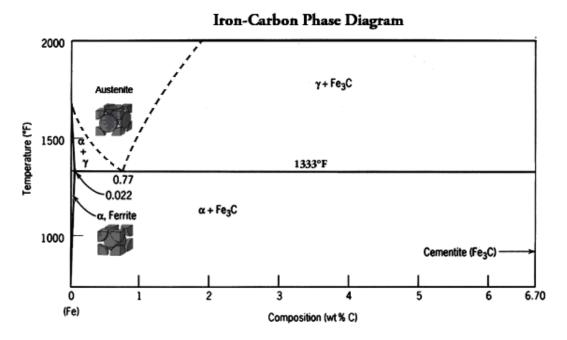
Figure 6.1: Iron-Carbon Phase Diagram
