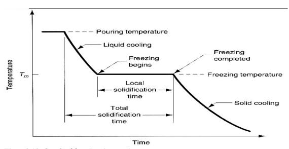
Figure 2.10: Graph of freezing time against temperature
