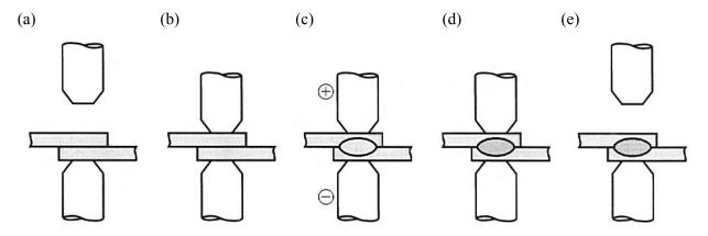
Figure 5.10: Steps in a spot welding cycle: (a) parts inserted between open electrodes, (b) electrodes close and force is applied, (c) weld time (current is switched), (d) current is turned off but force is maintained, and (e) electrodes are opened, and the welded assembly is removed.
