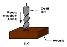
Figure 2.15: (a) Turning operation (b) Drilling operation
