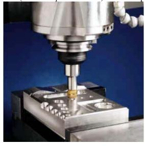
Figure 2.24: End milling operation used to cut a pocket in an aluminium work part.
