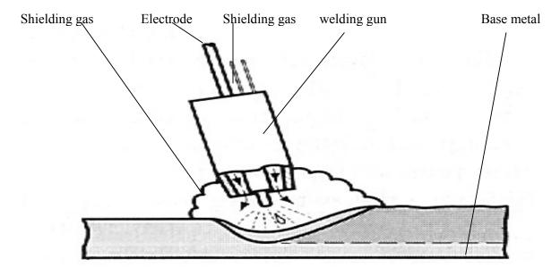
Figure 5.7: Gas metal arc welding operation.
