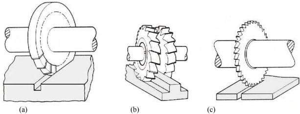
Figure 2.22: Peripheral milling operations with narrow cutters: (a) slotting, (b) straddle milling, and (c) slitting.
