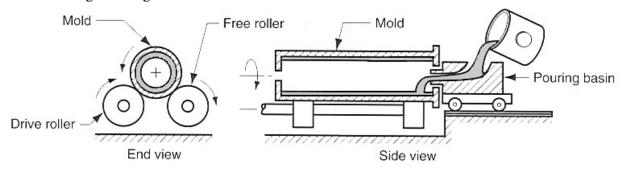
Figure 2.7: True horizontal centrifugal casting
