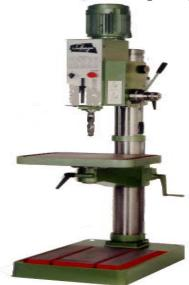
Figure 2.26: Drilling Machine
