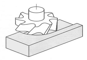
Figure 2.23: Partial face milling operation.
