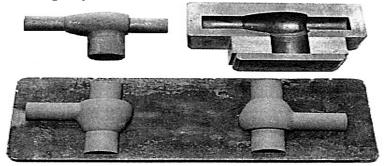
Figure 2.3: Cores used in casting
