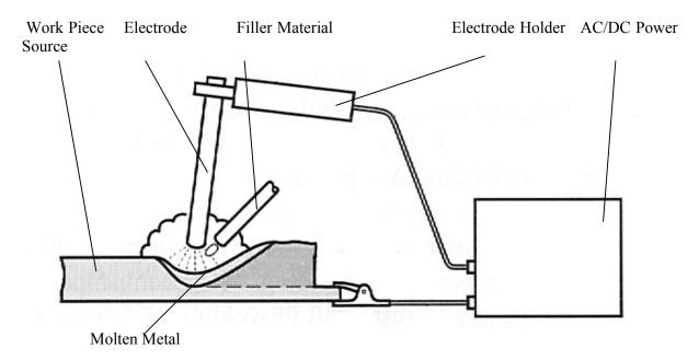
Figure 5.4: Arc Welding Operation
