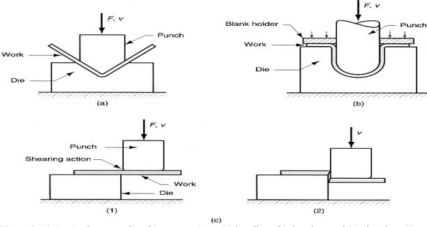
*Figure 2.14: Basic sheet metalworking operations*: (a) bending, (b) drawing, and (c) shearing; (1) as punch first contacts sheet and (2) after cutting. In the Figure, F and v indicate force and relative motion
