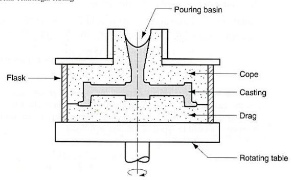
Figure 2.8: Semi-centrifugal casting
