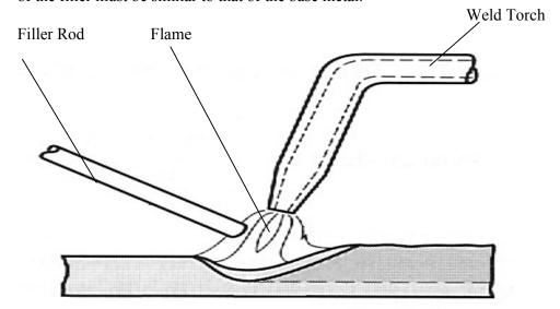
Figure 5.3: Oxyfuel gas welding operation.
