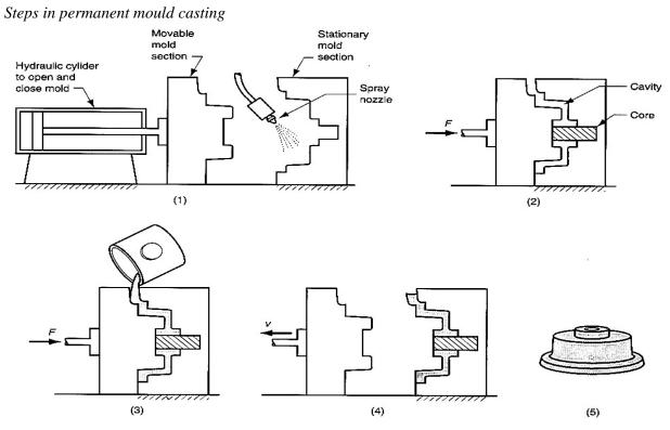
**Figure 2.6:** Steps in permanent mould casting: (1) mould is preheated and coated with lubricant for ease of separation of the casting; (2) cores (if used) are inserted and mould is closed; (3) molten metal is poured into the mould; and (4) mould is open and finished part removed. Finished part is shown in (5)
