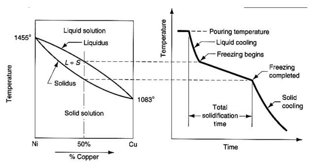
Figure 2.11: Freezing temperature of copper against time.
