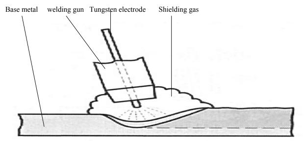
Figure 5.8: Gas tungsten arc welding operation.
