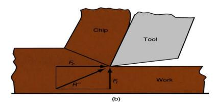
Figure 3.3: Forces in metal cutting: (b) forces acting on the tool that can be measured Source: Groover (2007)
