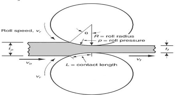
Figure 2.12: Flat rolling process
