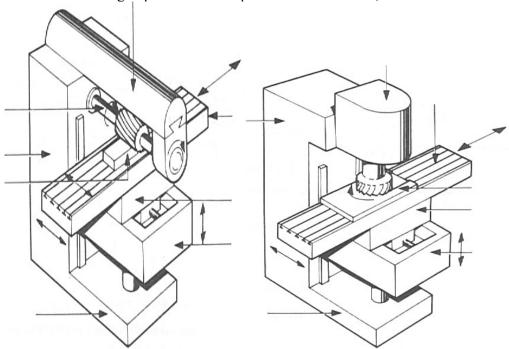
Figure 2.25: Two basic types of column-and-knee milling machines, (Left) horizontal and (Right) vertical.
