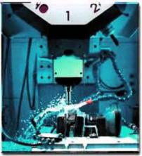
Figure 3.1: Application of flooding in milling
