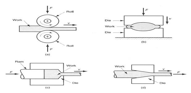
Figure 2.13: Types of Deformation processes
