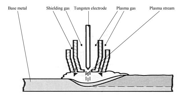
Figure 5.9: Plasma Arc Welding
