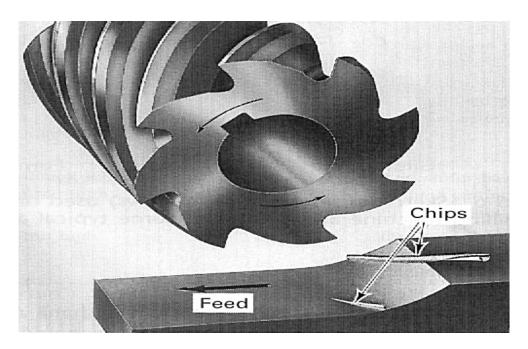
Figure 2.20: Milling operation.
