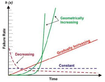
Depending upon machine type, the failure rate may decrease, remain constant, gradually increase or geometrically increase as a function of time
