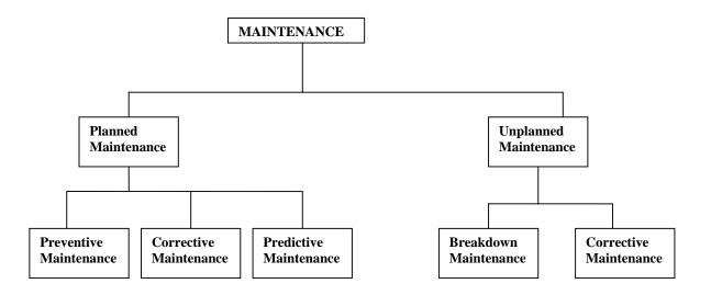
Figure 1: Diagrammatic representation of Types of Maintenance
