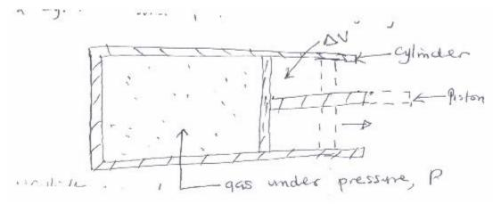
The work (dW) done by the gas when the piston moves to the right under pressure P such that the volume of the gas increases by dV is
