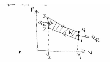
The net work produced by the engine is given by
