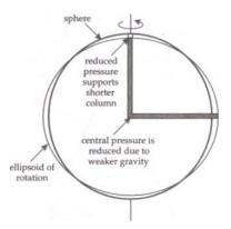
Newton's argument that the shape of the rotating Earth should be flattened at the poles and bulge at the equator was based on hydrostatic equilibrium between polar and equatorial pressure columns (after Strahler, 1963).
