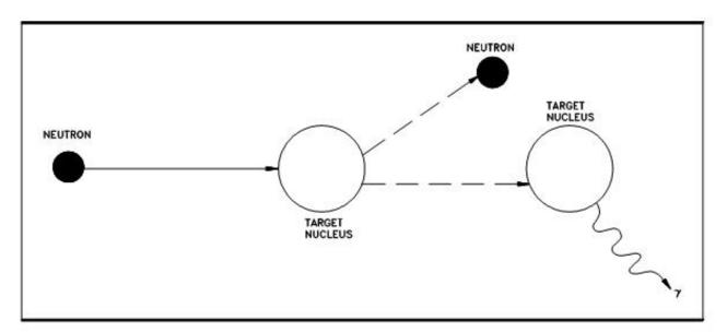
Figure 17 Inelastic Scattering
