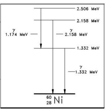
Figure 7 Energy Level Diagram - Nickel-60
