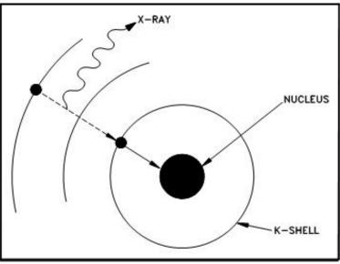
Figure 9 Orbital Electron Capture
