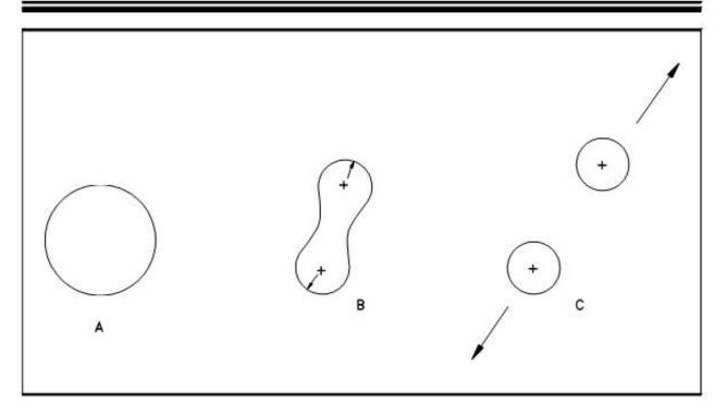
Figure 18 Liquid Drop Model of Fission
