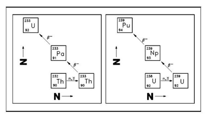
Figure 19 Conversion of Fertile Nuclides to Fissile Nuclides
