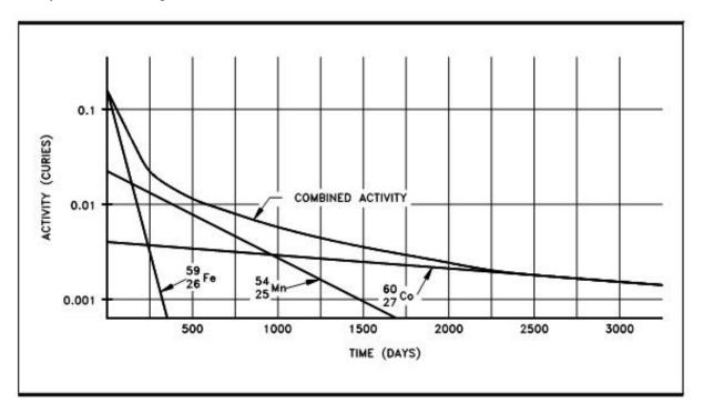
Figure 12 Combined Decay of Iron-56, Manganese-54, and Cobalt-60
