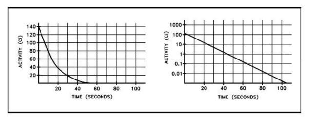
Figure 11 Linear and Semi-log Plots of Nitrogen-16 Decay
