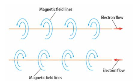
When electric current flows through a wire, a magnetic field forms around the wire. The direction of the magnetic field depends on the direction of the current in the wire.
