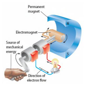
The electromagnet in a generator is rotated by some outside source of mechanical energy. In this setup, a student can rotate a crank to turn the electromagnet.
