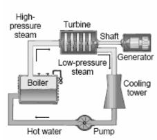
Fig. 9.4.3 - A steam turbine extracts work from steam as that steam flows from a high-pressure boiler to a low-pressure cooling tower. The cooling tower condenses the steam into hot water, which is then pumped back into the boiler.
