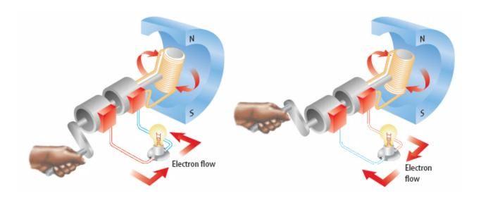
Therefore to generate electricity, all we really need to do is have some (mechanical) mechanism turn a crank that rotates a loop of wire between stationary magnets. The faster we can get this crank turned, the more current we can generate.
