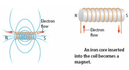
So now we know that a current can create a magnetic field. But can a magnetic field create a current flow? If so then we have a means of generating electricity.
