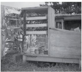
Fig. 1: Solar Incubator
