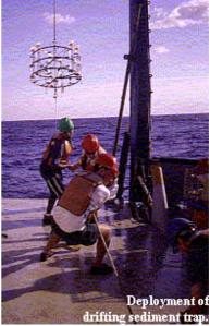
from the surface waters to the deep sea where it is eventually decomposed by bacteria. The sediment traps are attached to a line that has floats on the surface and a weight at the bottom to keep it vertical. Some sediment
