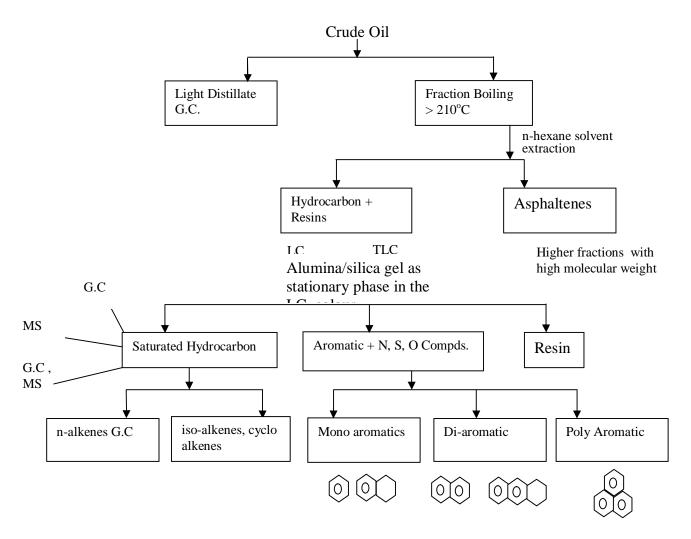
Fig 2: Analytical Procedure of Assay catalysis in chemical characterization of crude oil.
