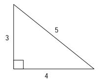
This fact can be used in setting out a right angle triangle with a chain, the length of the triangles of the multipliers of 3; 4:5.
