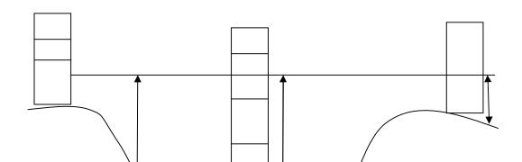
When two or more points are not on the same elevation, there is difference of level. Suppose this point level is held at an eye level of 1.5m, the horizontal plane at spirit level extended in imagination over the table, the plane will cut a rule held vertically on a rule hold at 0.75m at Mr. A, similarly if rule is held on chair at point C the reading at the interception of horizontal plane will be at 1.05m while the reading of rule held on the floor at Mr B will be 1.5m.
