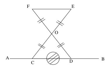
Fix a pole at C, O and E so that COE is a straight line and CO = OE. Also fix another set of pole D and F such that DOF is a straight line and Do = OF
