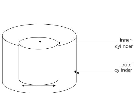
The very infiltration consist of a cylinder driver a fewer continue into the soil to prevent leakage. There are really two cylinder one inside the other and forming two concentric rings on the outside. The inner ring, which is usually 23cm in diameter is the one used to determine infiltration rate. The outer ring 36cm in diameter is meant to reduce the border effects on the inner rings.
