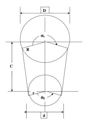
Figure 3. Geometry of Belt Drive
