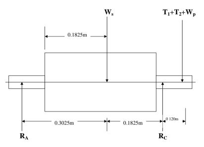
Figure 1 : Bending Loads on the Wormshaft
