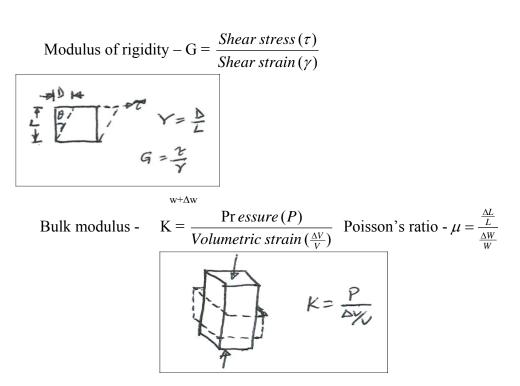
E = Elastic Modulus, G = Modulus of rigidity, K = Bulk Modulus,  $\mu$  = Poisson ratio  $\frac{1}{E} = \frac{1}{3G} + \frac{1}{9K}, \qquad E = 3K(1 - 2\mu), \qquad E = 2G(1 - \mu)$ Liquid is not compressible, hence G = 0 From Eqn 3, E =  $2x0(1-\mu) = 0$ Liquid doesn't support shear stress, this implies K =  $\infty$  In Eqn 2,  $\frac{E}{3\infty} = 0$  for E = 0 or K =  $\infty$ Hence  $1 - 2\mu = 0$ Therefore  $\mu = \frac{1}{2}$
