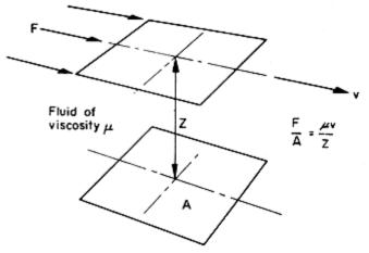
Figure 1. Viscous forces in a fluid.
