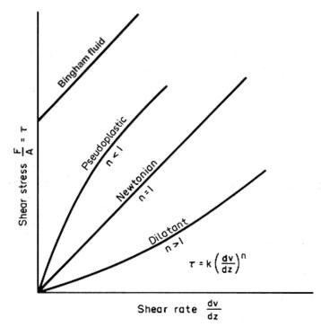
Figure 3.6. Shear stress/shear rate relationships in liquids.
