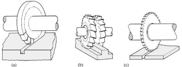
Figure 2.22: Peripheral milling operations with narrow cutters: (a) slotting, (b) straddle milling, and (c) slitting.
