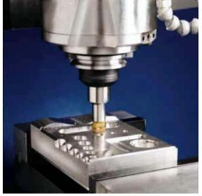
Figure 2.24: End milling operation used to cut a pocket in an aluminium work part.
