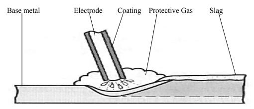
Figure 5.5: Shielded metal arc welding operation
