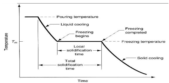
Figure 2.10: Graph of freezing time against temperature
