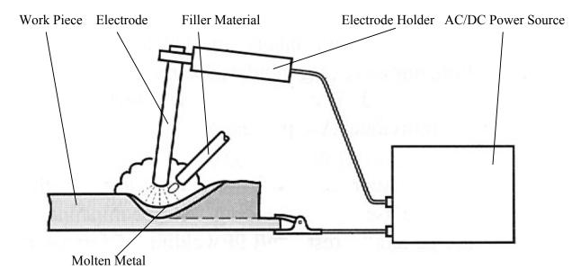
Figure 5.4: Arc Welding Operation
