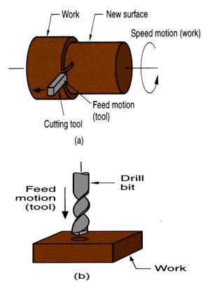
Figure 2.15: (a) Turning operation (b) Drilling operation Source: Groover (2007)
