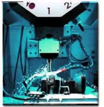
Figure 3.1: Application of flooding in milling
