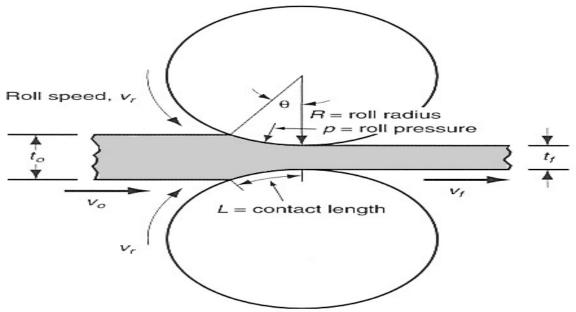
Figure 2.12: Flat rolling process
