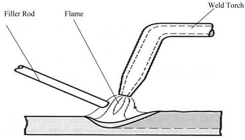
Figure 5.3: Oxyfuel gas welding operation.
