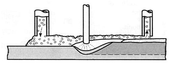
Figure 5.6: Submerged arc-welding operation.
