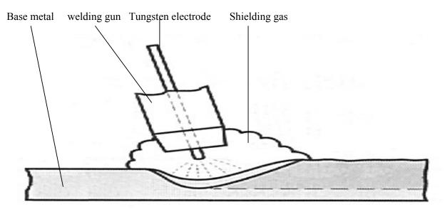
Figure 5.8: Gas tungsten arc welding operation.
