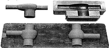
Figure 2.3: Cores used in casting
