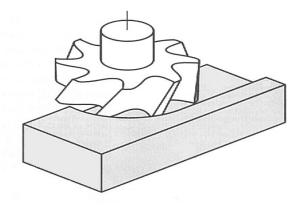
*Figure 2.23: Partial face milling operation.* The face-milling cutter machines only one side of the work piece.
