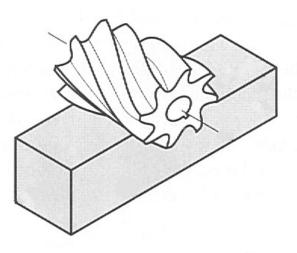
Figure 2.21: Peripheral slab milling operation
