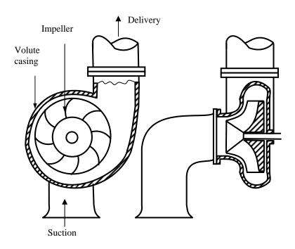
Fig. 4.1: Centrifugal pump
