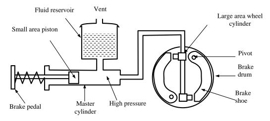
Fig. 5.7: Hydraulic Vehicle brakes
