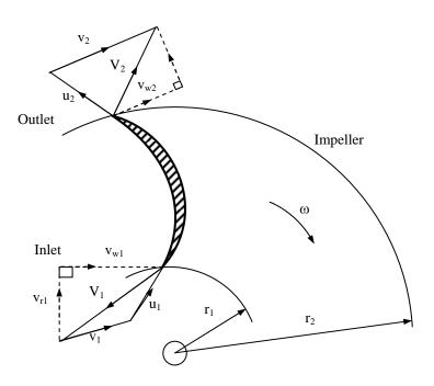
Fig. 4.2: Relative velocity triangles at inlet and outlet.
