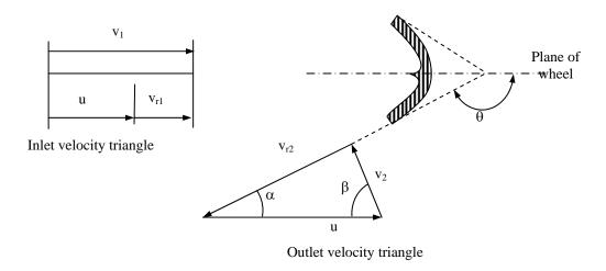
Fig. 3.4: Inlet and outlet velocity triangles.
