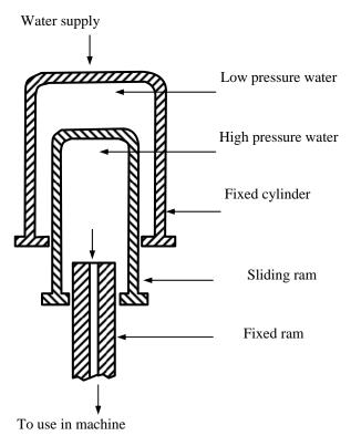
Fig. 5.6: Hydraulic intensifier
