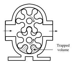
Fig. 5.4: Gear Pump
