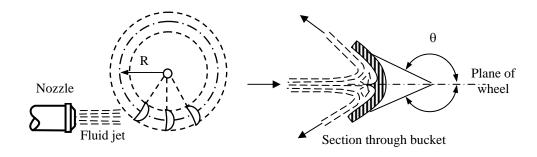
Fig. 3.3: Pelton wheel turbine.
