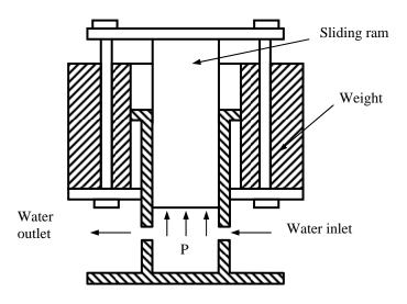
Fig. 5.5: Hydraulic accumulator
