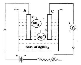
Here acqueous solution of AgNO<sub>3</sub> is used as an electrolyte and two plates A and C silver are partially immersed in it which are the electrodes. The electrodes are connected to a battery from which current enters the electrolyte through A and leaves through C.
