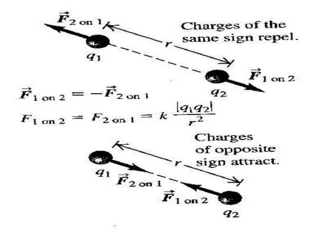
The force on each charge is along the line joining the two charges - repulsive if  $q_1$  and  $q_2$  have the same sign, attractive if they have opposite signs. The forces form an action-
