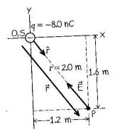
The distance from the charge at the source point S (which in this example is at the origin 0) to the field point P is:  $r = \sqrt{x^2 + y^2} = \sqrt{(1.2m)^2 + (-1.6m)^2} = 2.0m$
