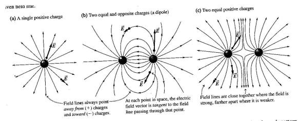
The actual field vectors have been drawn at several points in each pattern. Notice that in general, the magnitude of the electric field is different at different points on a given field line; a field line is not a curve of constant electric –field magnitude!
