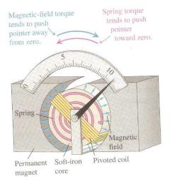
Thus, the angular deflection of the coil and pointer is directly proportional to the coil current, and the device can be calibrated to measure current.
