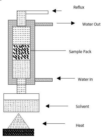
A round flask is used for the solvent. Heat is supplied with an electric plate and water recirculated to maintain a constant temperature during the extraction process (Figure 2.2). Extraction is performed using solvents such as petroleum ether, benzene, diethyl ether, etc., a process that takes between 4-6 h. After the extraction, the oil is recovered from the flask through evaporation of the water at 105°C in an oven until constant weight is achieved.
