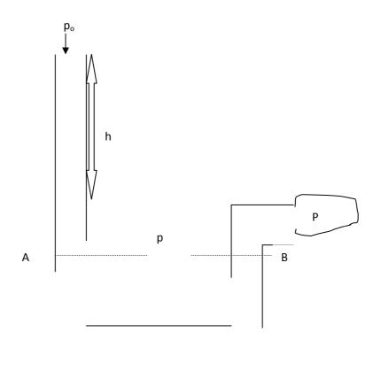
It consists essentially of a U-shaped tube containing a liquid (usually mercury or water), one arm of which is open to the atmosphere, the other being connected to the vessel whose pressure we wish to measure. If the manometer shows the liquid in open arm at a height h above that in the closed arm, the pressure in the open arm at A is equal to that of the closed arm at B. Considering the open arm, we get
