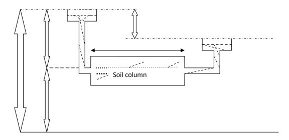
A steady flow of water is occurring from left to right, from an upper reservoir to a lower one, in each of which the water level is maintained constant. The discharge rate, Q, being the volume V flowing through the column per unit time is directly proportional to the cross-sectional area and to the hydraulic head drop  $\Delta H$ , and inversely proportional to the length of the column:
