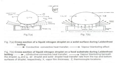
$$\lambda \rho_1 \frac{V_o}{t_f} = h_{av} A_{av} \Delta T_{mn}$$
