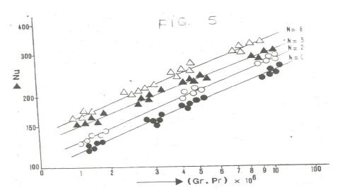
Fig. 14: The variations of Nusselt number (Nu) with Rayleigh number (Ra) as influenced by the number of mixing/stirring (N) of the paste during reconstitution
