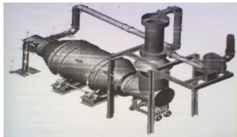
Fig. 8: Construction of Rotary Furnace
