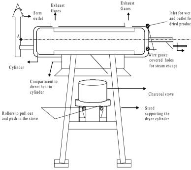
Fig. 7: UNAAB Fufu Rotary Drier
