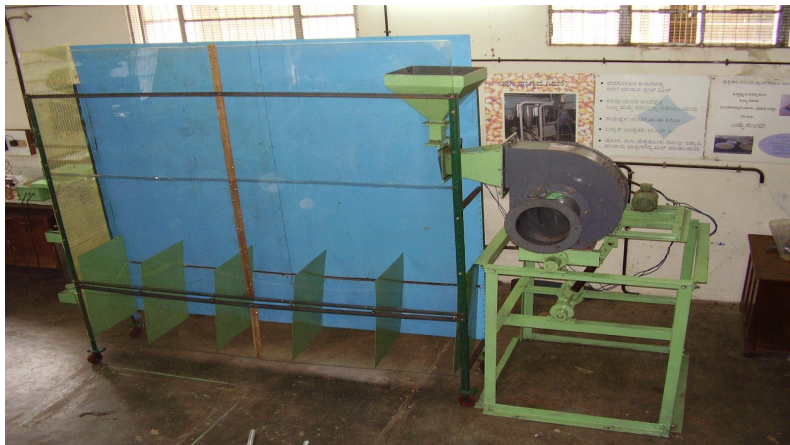
Fig. 20: The assembly of the cross flow test rig with the feed hopper (without the collection trays)
