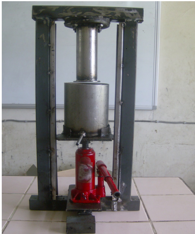
Fig. 16: Picture of the Hydraulic Oil Extractor Showing the Cage Casing and Discharge Chute
