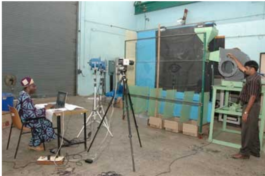
Fig. 21: A typical arrangement for an horizontal air flow experiment using high speed camera
