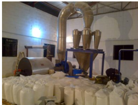
Plate 10: NOBEX Flash Dryer in Oamsal SME, Ayede Ekiti, Nigeria Source: Sanni and Siwoku (2014).
