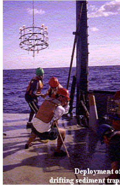
Deployment of drifting sediment trap.
