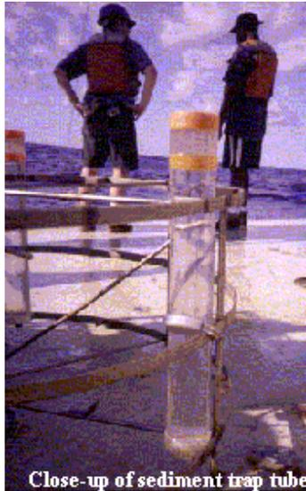
Close-up of sediment trap tube
