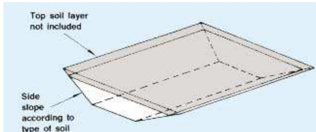
For reasonably flat, level surfaces, where *excavated width is at least 30 times the depth*, volume of excavation can be estimated as:
