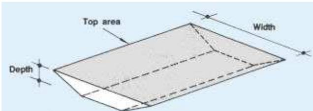
$$V = \text{top area} \times \text{depth of excavation.}$$
