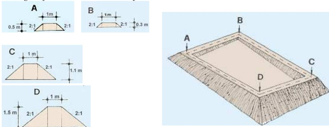
For a more accurate measurement of dike volume on rough ground, you should apply the following formula, known as Simpson's rule, where:  $V = (d \div 3) \times [A_1 + A_n + 4(A_2 + A_4 + \dots + A_{n-1}) + 2(A_3 + A_5 + \dots + A_{n-2})]$ . Proceed as follows:
