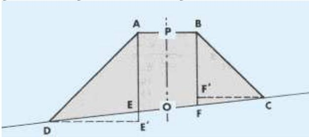
*Calculating the cross-section of a dike on irregular ground using a scale drawing*
