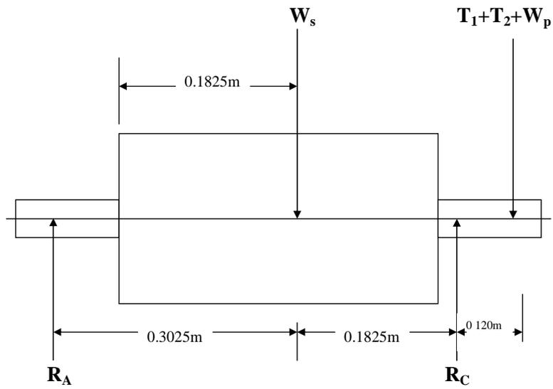
**Figure 1 : Bending Loads on the Wormshaft**
