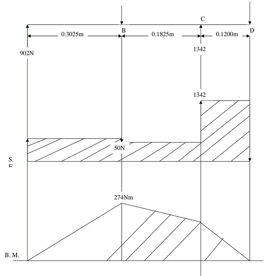
**Figure 4.19: Shear Force and Bending Moment Diagrams**
