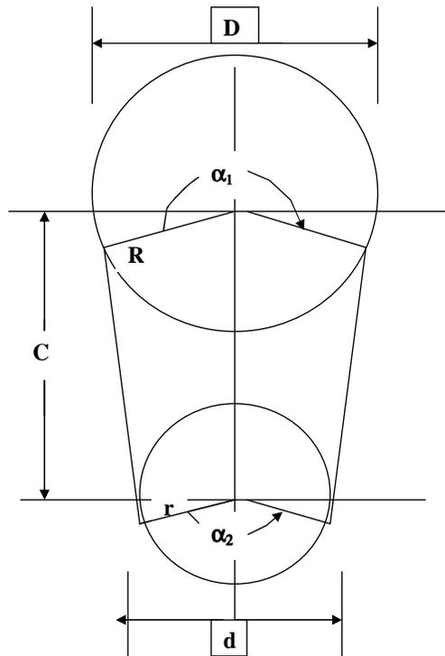
Figure 3. Geometry of Belt Drive
