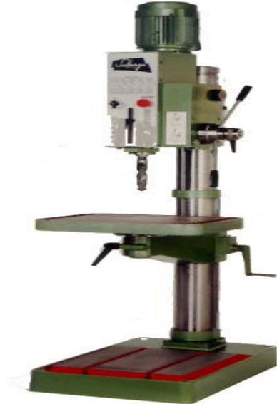
**Figure 2.26: Drilling Machine**
