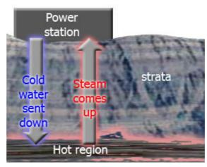
Hot rocks underground heat water to produce steam. We drill holes down to the hot region, steam comes up, is purified and used to drive turbines, which drive electric generators.
