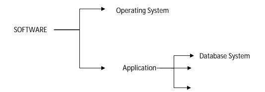
Database system is designed to handle data store in a database. This system is to update and retrieve information stored in the database when request are issued. During database operation, the operating system would load database system and application program. The application program can execute any instruction until it wants data from database. At this point, the database
