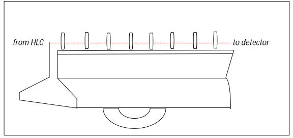
The flame is like a cell of ground state atoms which absorb resonance line from the hollow cathode lamp while the rest of the signal goes on to the detector which measures the absorbance.
