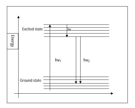
The molecules emit energy hv by collision and drops to the lowest vibrational level of the excited state. The probability of return to ground state with emission of photon is greatest at
