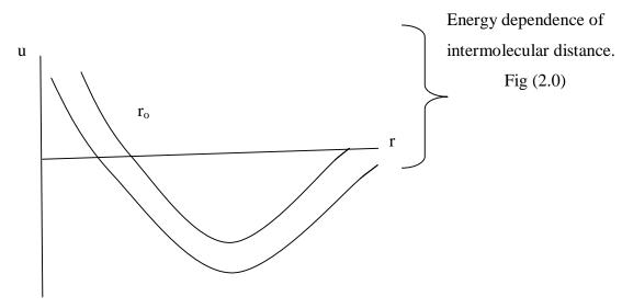
**Note**: That the molecules are normally at freed position (distance  $r_o$  from one another) and their forces in any molecule is zero; and potential energy (p.e) is minimum.
