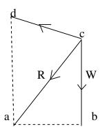
Forces ab and ad can be replaced completely by a single force Ac i.e. to replace a single force by two other forces in any convenient direction. These two forces are known as the Components of the single force.
