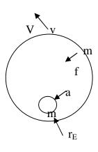
m = mass of satellite r = sum of the Earth's radius  $r_E$  plus the satellite's height h above the Earth:  $r = r_E$  th  $V_v = velocity$  of the orbit
