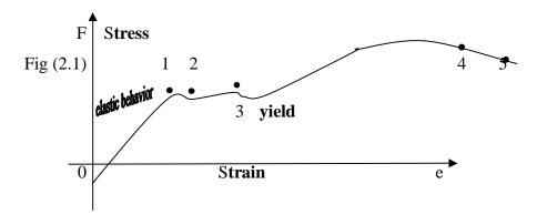
0-2, wire return to its original length after the load had been removed. 2, is known as elastic limit. After this print, it is brittle. 3, is the yield print beyond this print, extension is rapid, and this known as plasticity. At 4, material is under maximum force or stress that can be sustained. At 5, it is the breaking point.
