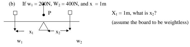
**Solution:** First law of equilibrium condition, N force exerted by the support must balance their weights such that the net force is zero.
