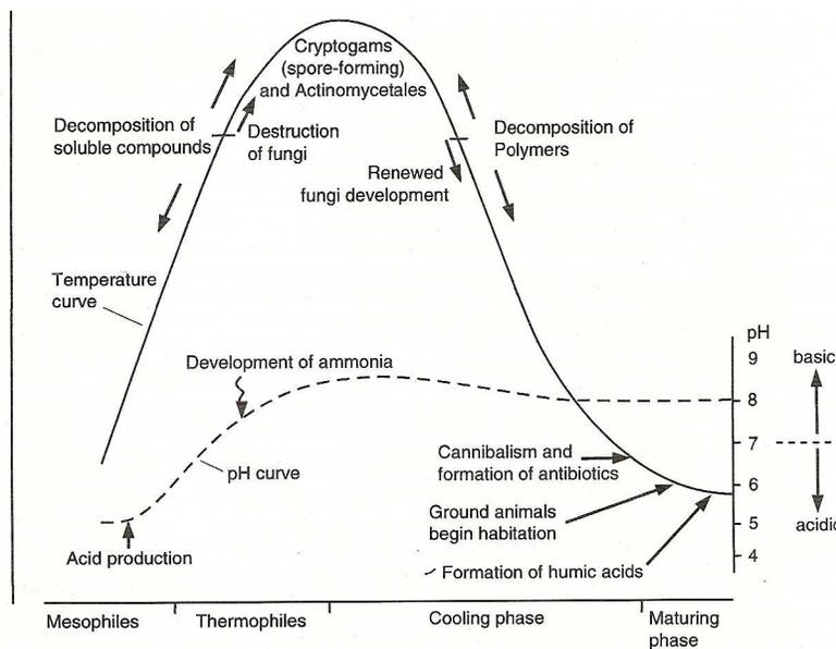
Figure 1: Temperature and pH changes with associated processes during composting (Muller-Shannan and Kotschi, 1994)
