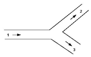
(c) If pipe 1 diameter = 50mm, mean velocity 2m/s, pipe 2 diameter (40mm) takes 30% of
