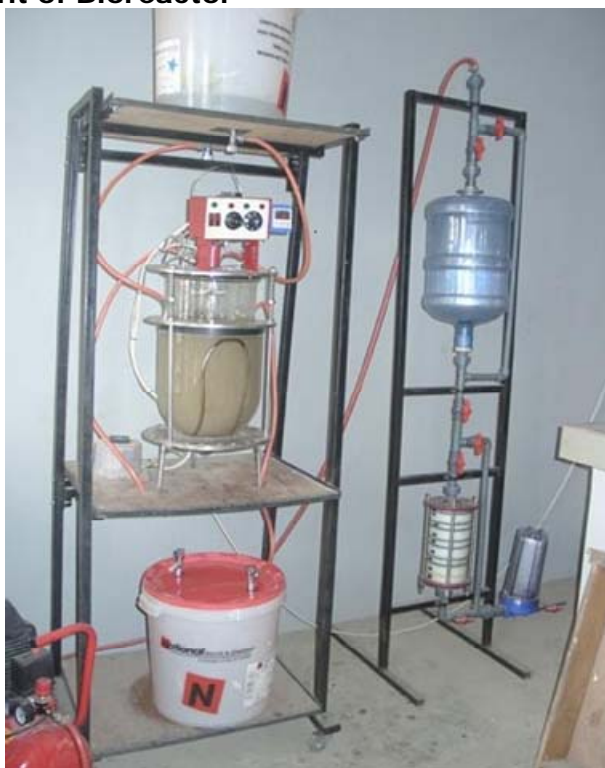
A 10 LITRE GLASS BIOREACTOR + FILTER UNIT DESIGNED AND FABRICATED IN MY LABORATORY
