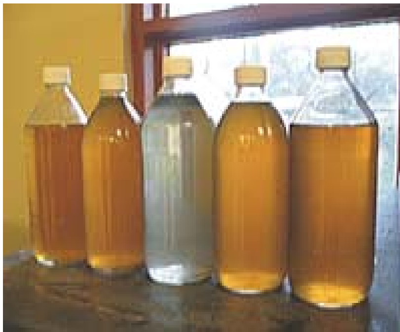
GLUCOSE SYRUP FROM CASSAVA PRODUCED IN MY LABORATORY DECOLOURISED USING ACTIVATED CHARCOAL
