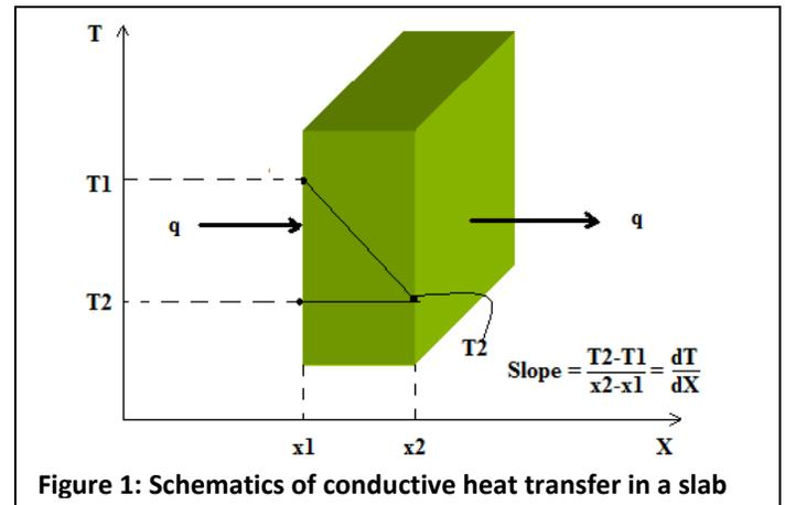
Figure 1: Schematics of conductive heat transfer in a slab
