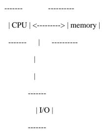
CPU -- controls the running of programs, executes instructions, makes requests of the memory. CPU stands for central processing unit.
