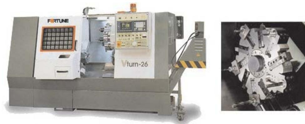
**Figure 2.18: CNC Lathe Machine**
