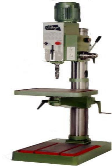
**Figure 2.26: Drilling Machine**
