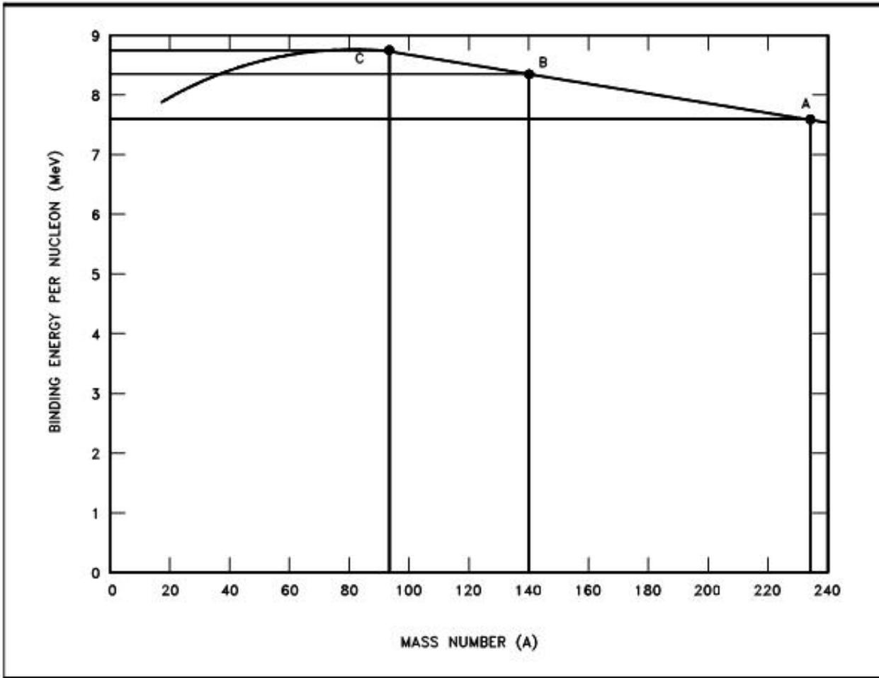
Figure 22 Change in Binding Energy for Typical Fission
