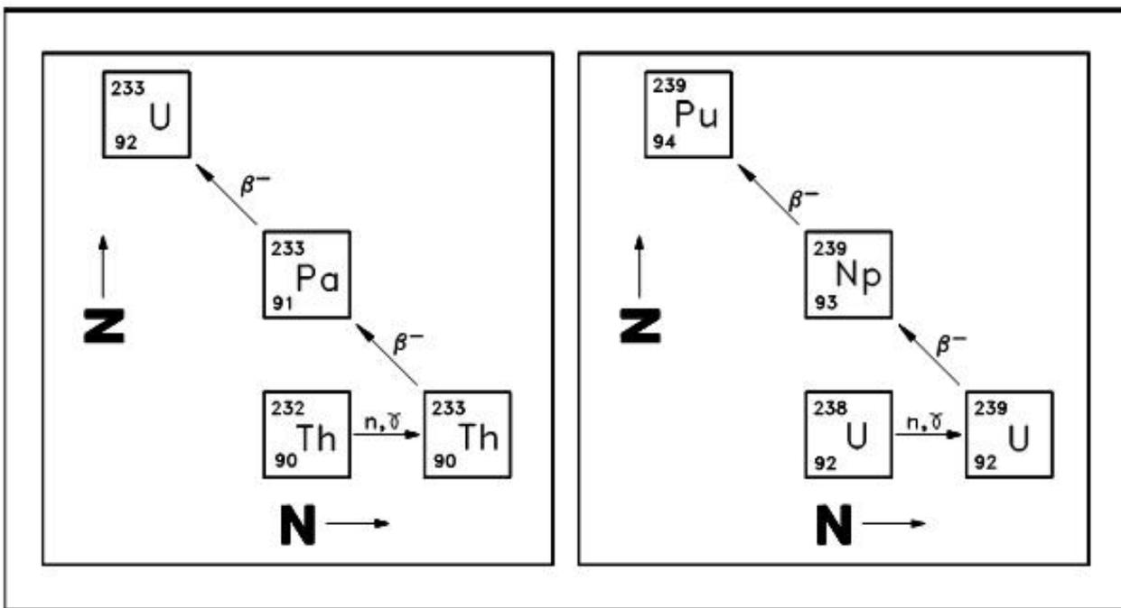
Figure 19 Conversion of Fertile Nuclides to Fissile Nuclides
