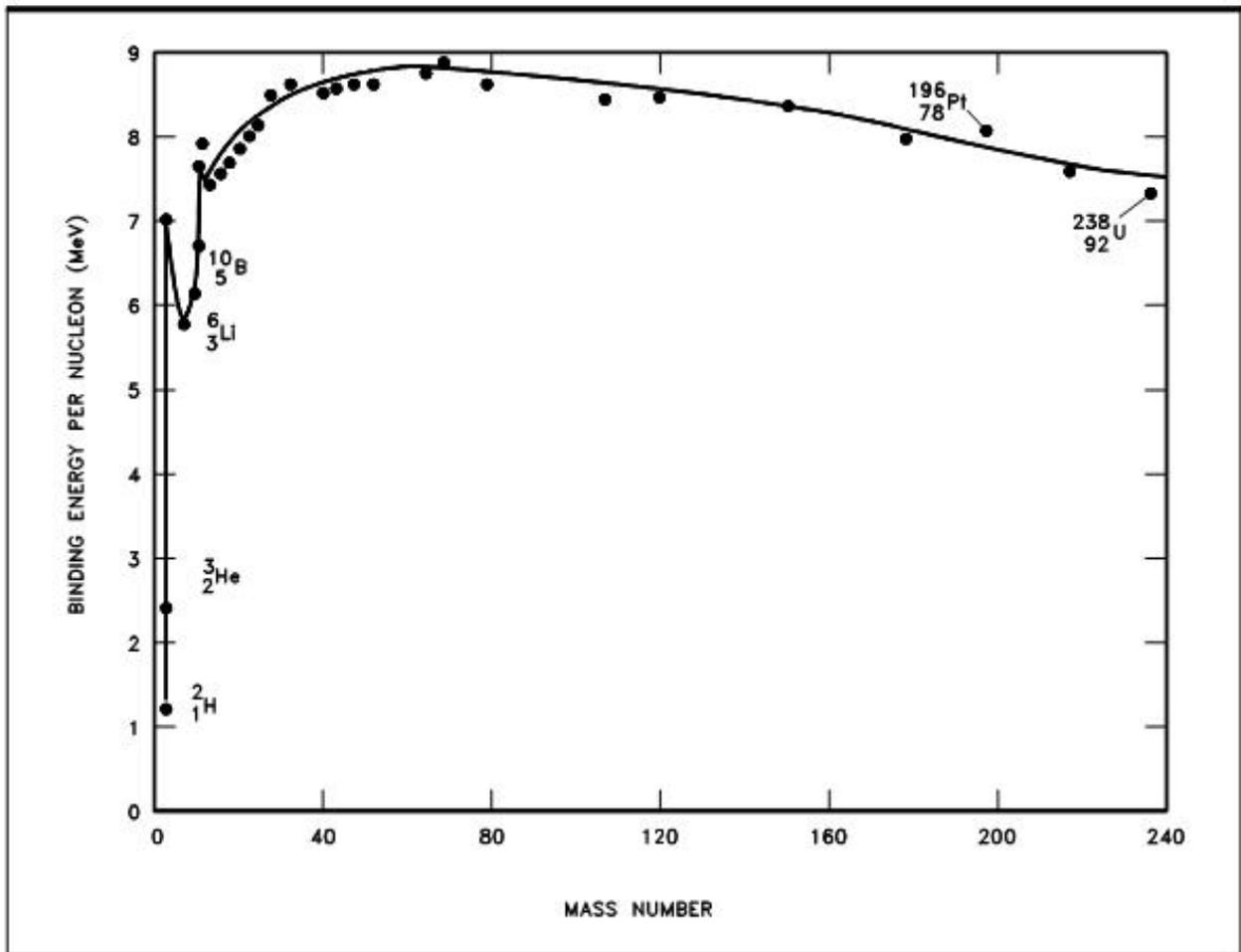
Figure 20 Binding Energy per Nucleon vs. Mass Number
