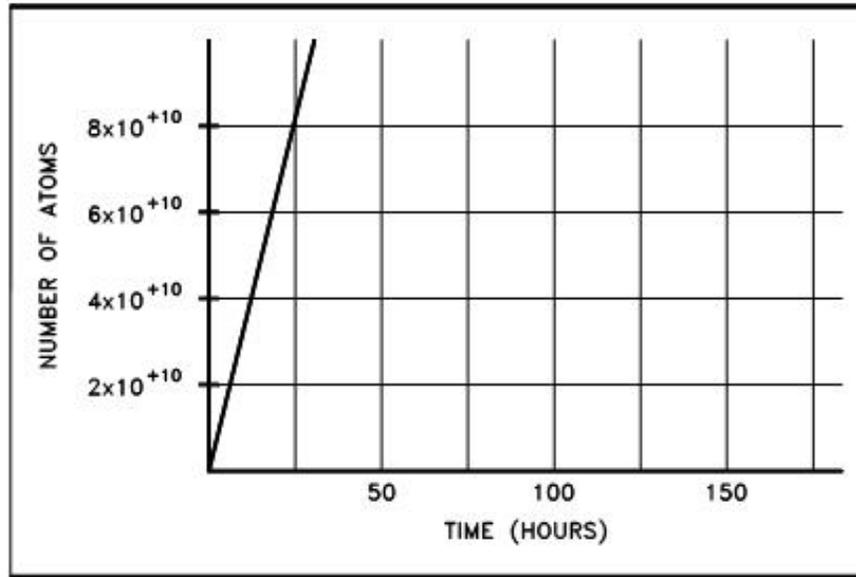
Figure 13 Cumulative Production of Sodium-24 Over Time
