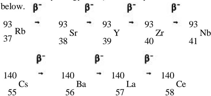
The energy released during the decay for each chain will be equivalent to the mass difference between the original fission product and the sum of the final stable nuclide and the beta particles emitted.
