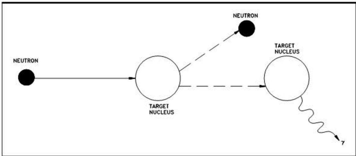
Figure 17 Inelastic Scattering
