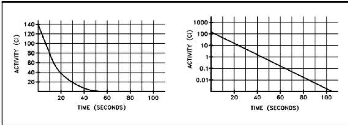
Figure 11 Linear and Semi-log Plots of Nitrogen-16 Decay
