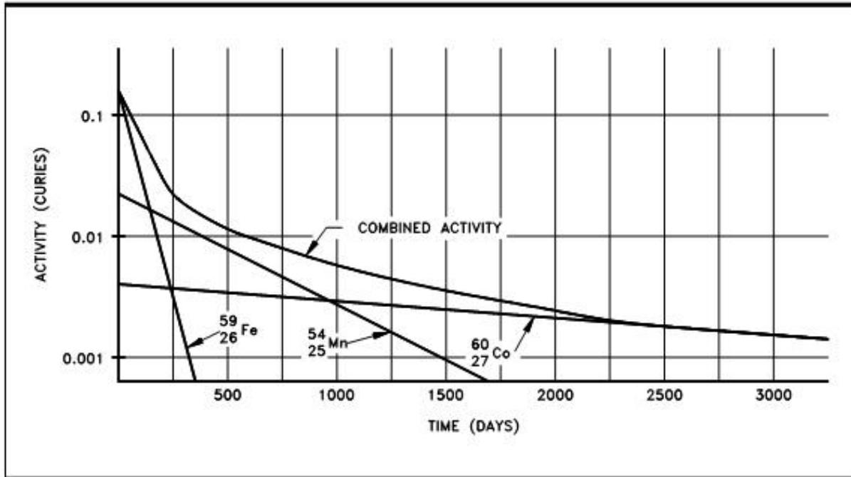
Figure 12 Combined Decay of Iron-56, Manganese-54, and Cobalt-60
