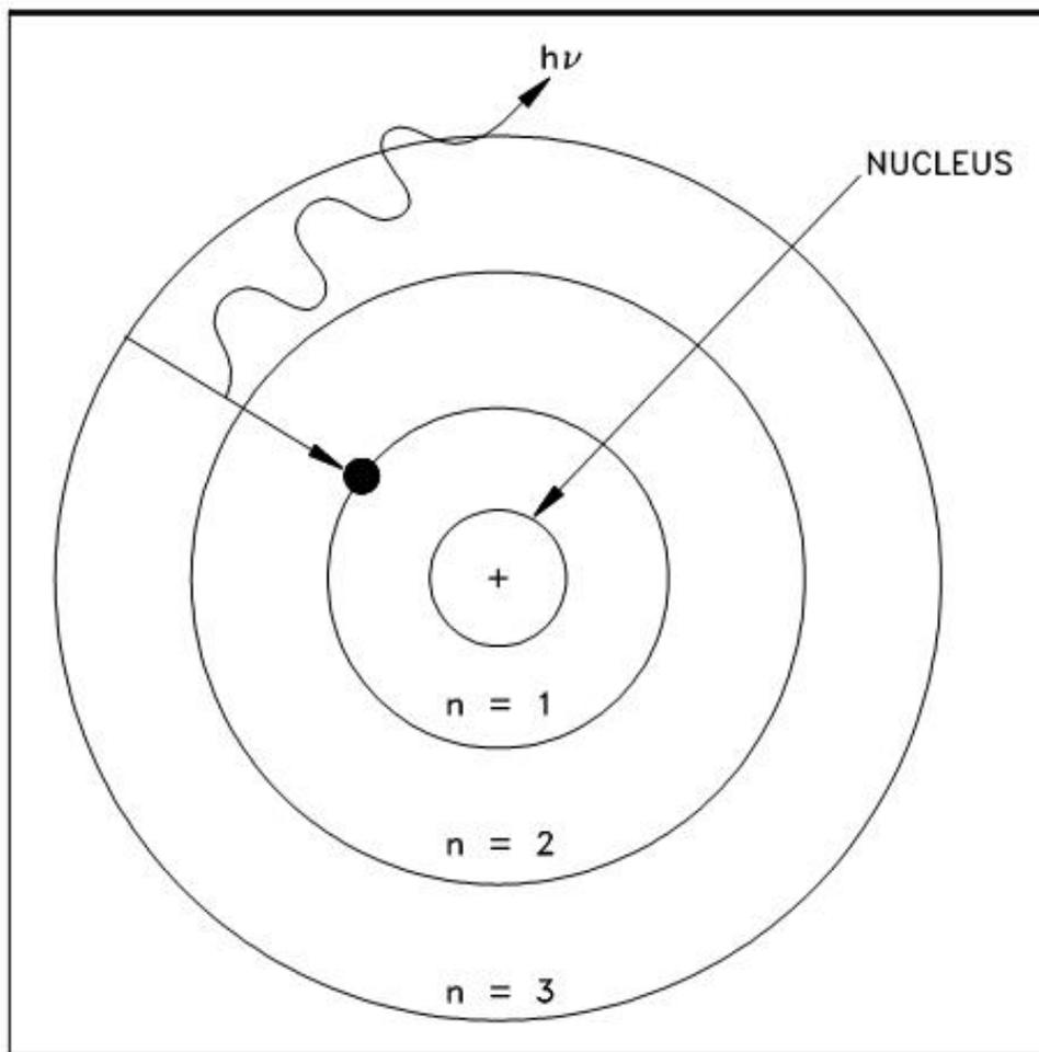
Figure 1 Bohr's Model of the Hydrogen Atom
