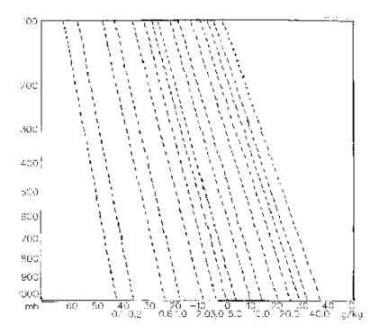
We can also determine the actual mixing ratio of the air parcel from this same set of lines if the dewpoint temperature were known also. If we know the pressure and both the air and dewpoint temperatures, we can determine the saturation mixing ratio and w, respectively. Thus, from the above example of an air parcel with  $T = 26^{\circ}C$  and P = 1000 mb, and a dewpoint, Td equal to  $15^{\circ}C$ , then the saturation mixing ratio is 20 g/kg and actual mixing ratio = 10 g/kg.
