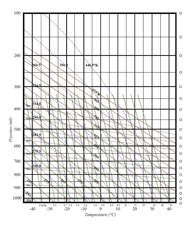
To find the temperature of a parcel: To find the temperature of a parcel lifted dry adiabatically, find the initial point (given temperature and pressure) and travel upwards parallel to the nearest dry adiabat. Since the wet adiabats diverge with decreasing pressure, when lifting a parcel wet adiabatically it is important to stay equidistant between two wet adiabats. *Do not go parallel to just one!*
