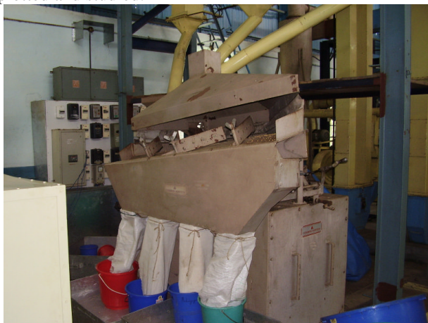
Fig. 2: Specific gravity separator at CFTRI 1 ton/day pilot maize mill
