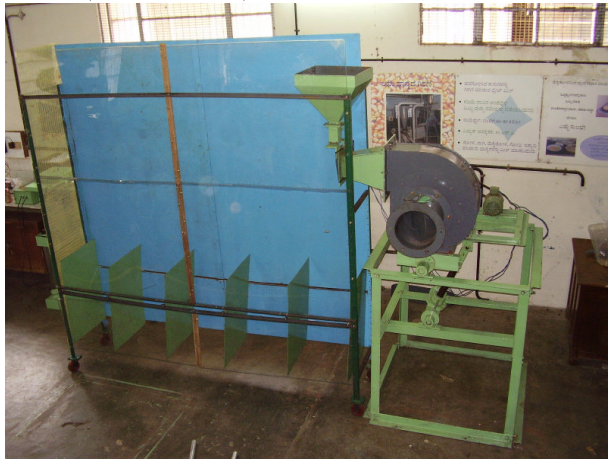
Fig. 1: The assembly of the cross flow test rig with the feed hopper (without the collection trays)
