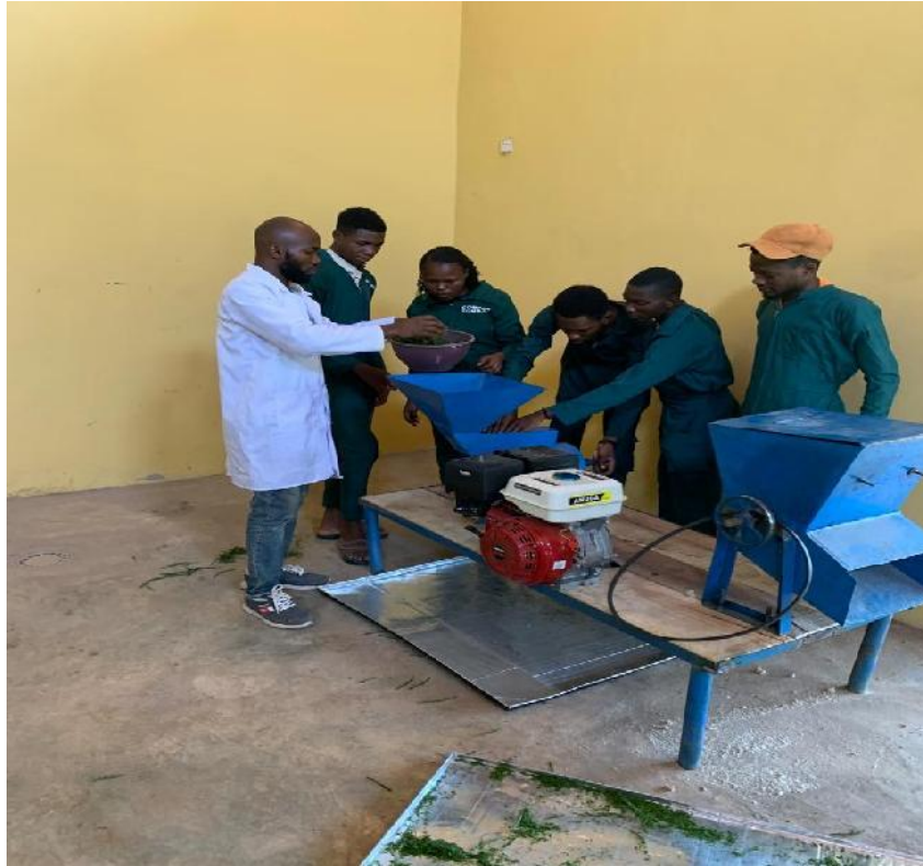
Picture. 1: Dr. Tolu Adebowale demonstrating the use of a combined cassava peel Grater and Grinder to Students
