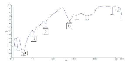
Fig. 6FT-IR spectrum of modified natural rubber latex (Akinlabi et. al. 2011).
