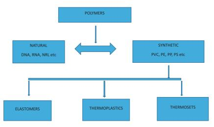
Fig. 1: Showing classification of polymers
