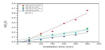
Figure 9 Effect of composites on Kinetics of photodegradation of methyl orange dye at pH 4.1. (Akinlabi *et. al.*, 2019)
