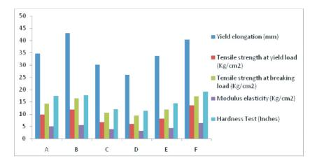
Fig. 22 : Physico- mechanical properties of vulcanisates(Akinlabi *et al* 2007)
