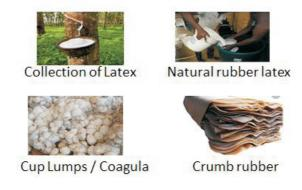
Figure 2 showing pictures of latex, cup lumps. Coagula and crumb rubber
