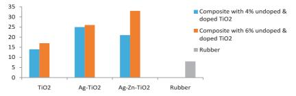
Figure 8 Photodegradation of methyl orange dye by composite filled with or without catalyst at pH 4.1 (Akinlabi *et. al.*, 2019)
