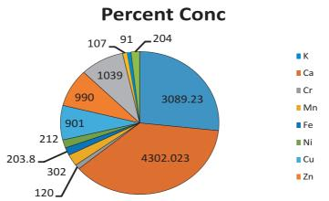
Fig. 21. Elemental composition of hydroxylated banana fibre(Akinlabi et al 2007)
