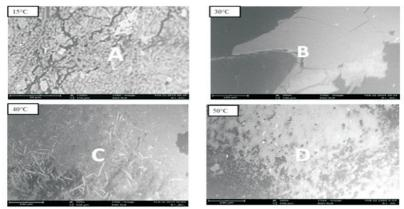
Fig. 10SEM micrographs of insulin biomembrane polymerised at different temperature (Akinlabi *et. al.*, 2019)
