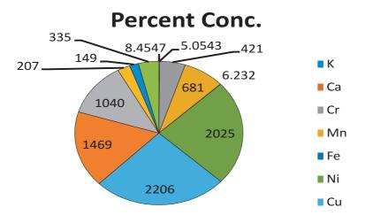
Fig. 20 Elemental composition of unmodified banana fibre(Akinlabi et al 2007)
