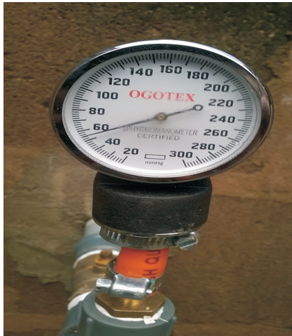
Plate 3: Pressure gauge for gas quantity determination
