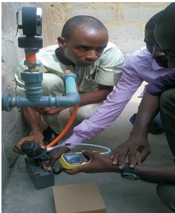
Plate 6: Measurement of gas flow rate
